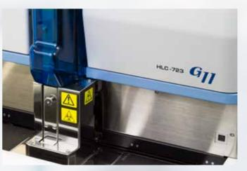
"What I find user friendly is the rack rotation switch. In this way the analyser knows when the last sample has been analysed and will go directly in wash mode. Afterwards there is a customisable timer to power off the analyser."
