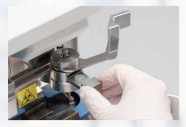
"Filter change is done in 2 seconds. Simply open the unit and replace the filter. It is a single action and replacing it, has so many benefits. My column will last longer and it ensures good quality results."
